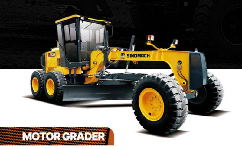
713H 717H 724H Operating Weight 37.200 KG 12.000 KG 23.500 KG Diesel Engine Weichai wp10g178E25 Cummins NT855-C280S10 Cummins NT855-C280S10 Rated Power 97 KW@2.200 RPM 175 KW/1.800 RPM 257 KW/2.000 RPM Moldboard 3.658 MM x 580 MM 560 MM 560 MM Blade 3.658 MM Planetary Gear Planetary Gear 17.5-25-12PR L-3 Tyre 3.725 MM 4.130 MM Transmission System 6 FW / 3 RW Single / Three Shank Single / Three Shank
